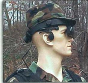
**The equipment needed to control a tactical mobile robot is wearable and part of a soldier's combat uniform. When activated, the gloves control movement, and a display in the glasses is connected to a camera mounted on the robot.** (Raytheon photos)
